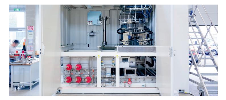
In five steps, the ionic compressor compresses gaseous hydrogen up to 90 MPa. On its piston is the eponymous ionic liquid which, however, does not bond with the gas. This liquid acts both as a lubricant and coolant and thus significantly reduces wear, because the ionic compressor has a lot less moving parts than a classic piston compressor. On top of that, it increases the compressor's energy efficiency due to better cooling and the avoidance of dead spots during the compression process.
